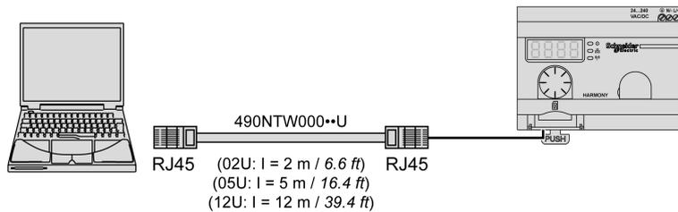
ZBRN2 access point is connected to the PC as shown in the following figure:
