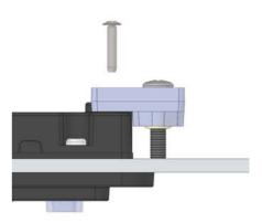
3. Tighten the M3 screws (#1 PZ) to attach each bracket to the rear of the unit.
