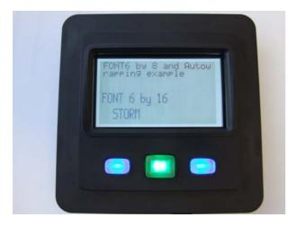
In above example, displays a mixture of fonts line 0 and 1 is using FONT6X8 and line 4 and 7 using FONT6X16.
