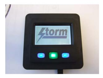
In above example, a "Storm" bitmap is loaded from the host application.
