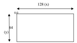
The USB Display has dedicated screen buffer (128 X 64) and it is this screen buffer holds the pixel image, before it is transfered to the LCD display. This allows the developer to first build up a image and then display it using the LCDFunction (SCREEN\_DISPLAY) command.
