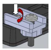
4. Tighten the M4 screws (#2 PZ) to pull the unit down to the panel surface
