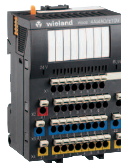
ricos 4AI4AO/±10 V 4 inputs and 4 outputs \pm 10 V Approvals:
