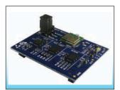
One development module, three standards: Bluetooth Classic, Bluetooth Low Energy and ANT™. This unique triple mode ETU – that's ETU for "Easy-To-Use" – module plugs directly into Panasonic Development Kits, Texas
