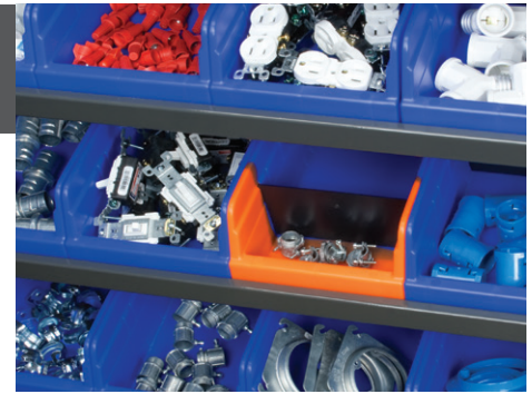
A complete Kanban system in a single bin The orange side indicates when supplies need to be replenished
