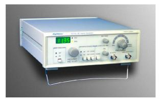
The *digimess*<sup>®</sup> SG100 is a very competitively priced microprocessor controlled RF signal generator. The unit covers the frequency 100kHz to 150MHz ( 450MHz 3rd harmonic ) in 6 ranges. A fine adjust control allows precise frequency selection and the set frequency is displayed by a 4 digit LED readout. The generator also includes both internal and external AM and FM modulation as well as an audio signal output. The SG100 is supplied with operating manual and mains lead.
