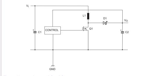
Fig 3. Non-synchronous DC-to-DC step-up converter
