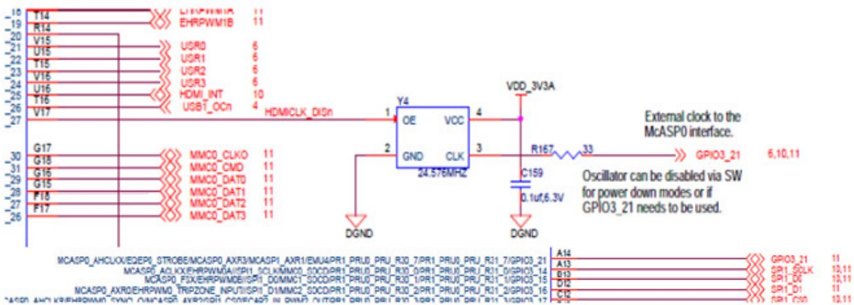
Figure 45 24.576MHz Oscillator
