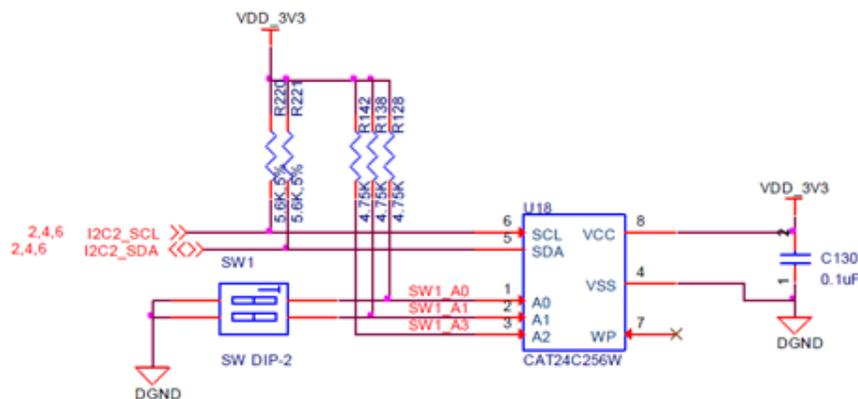
Figure 61 Expansion Board EEPROM Without Write Protect
