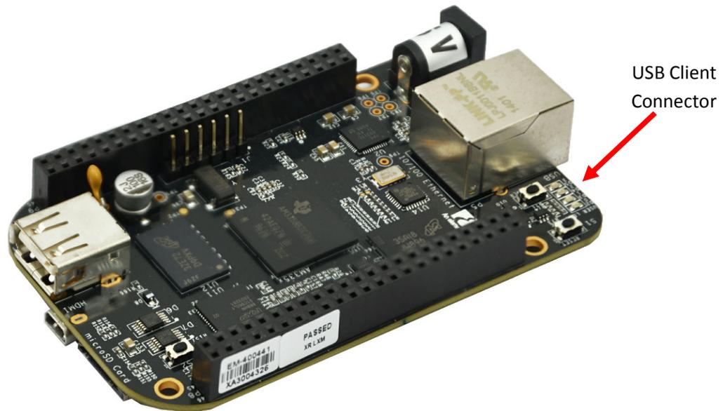
Figure 52 USB Client Connector
