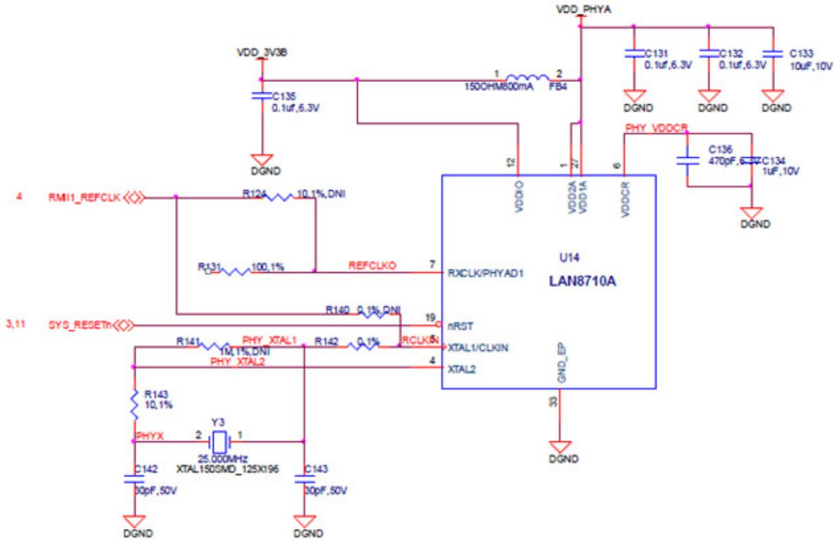
Figure 42 Ethernet. PHY, Power, Reset and Clocks
