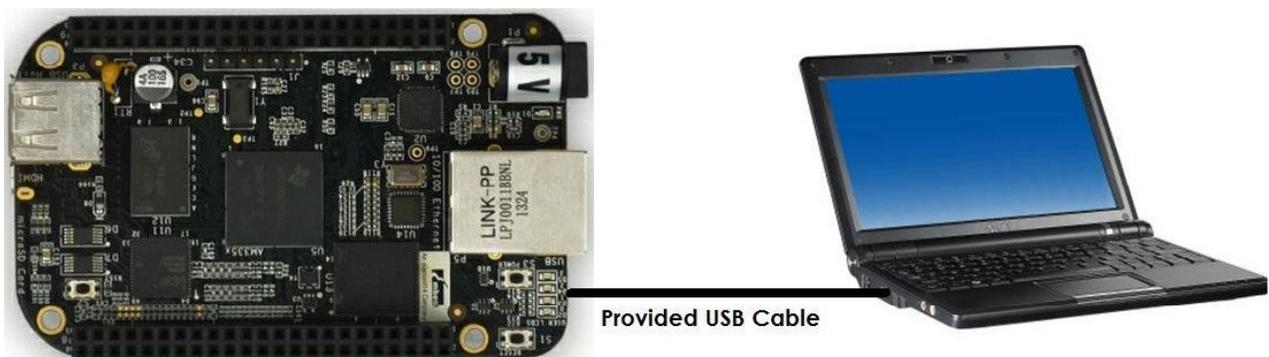
Figure 2 Tethered Configuration
