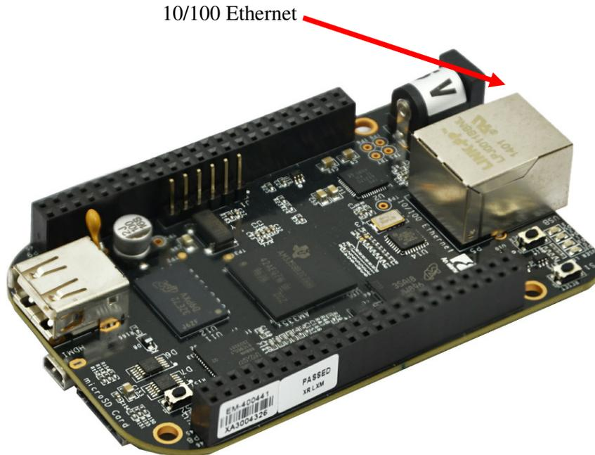
Figure 60 Ethernet Connector
