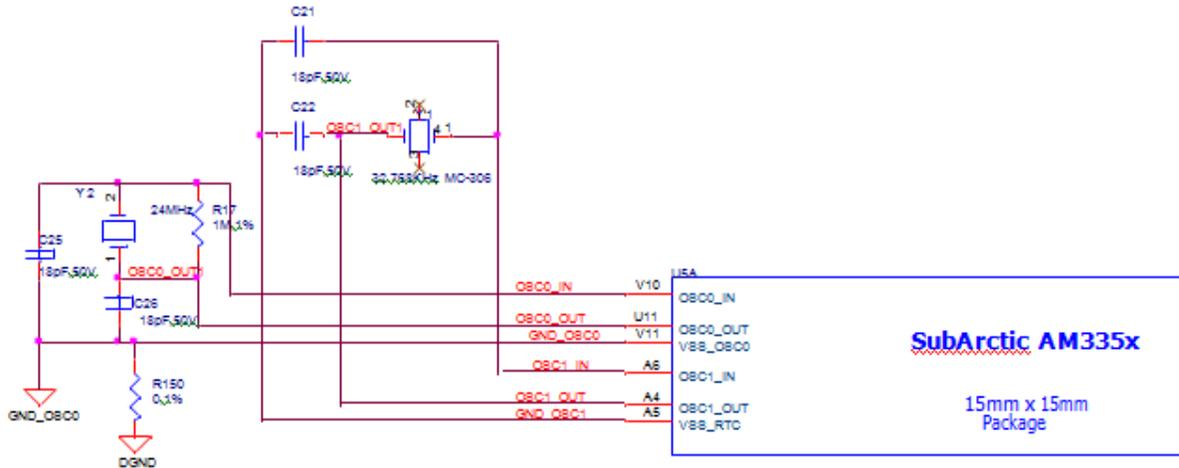
Figure 30 Processor Crystals
