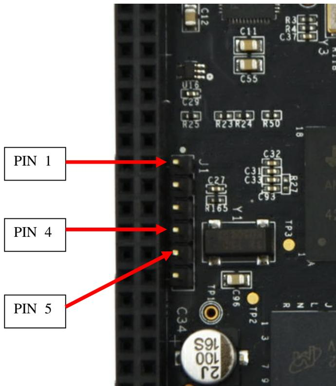
Figure 56 Serial connector
