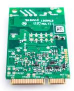
The Kvaser Mini PCI Express HS is a Card of type F2 (Full-Mini with bottom side keep outs).
