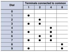
Note: The solid dot ● indicates that the internal switch is ON (i.e., connected to the common terminal).
