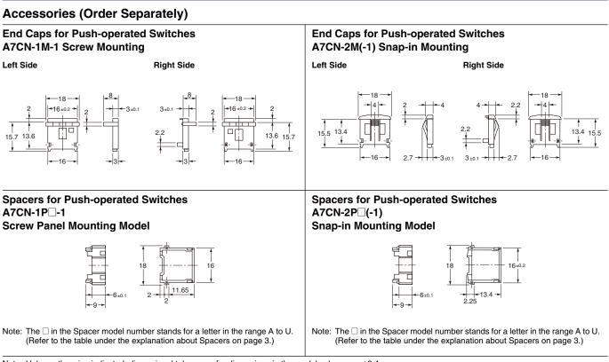
Note: Unless otherwise indicated, dimensional tolerances for dimensions in the models above are ±0.4mm.
