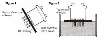
Using a Soldering Iron
