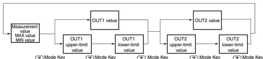
**Note:** When a comparative value is displayed, it can be changed by pressing the Shift Key and the Up Key (when key protection is OFF).
