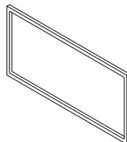
If the rubber packing is lost or damaged, it can be ordered using the following model number: K32-P1.
