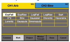
All models in the 4060 series provide non-volatile memory to create, store, and recall up to 24 different 16-kpt arbitrary waveforms and up to 8 different 512-kpt arbitrary waveforms. Users can also output any of the 36 built-in predefined arbitrary waveforms.
