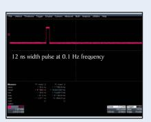
Unlike traditional DDS generators, the 4060 Series has the capability to output a rapid pulse at very low frequencies. Duty cycle can be set to as low as 0.0001%.
