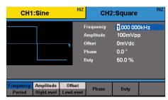
Large 4.3" color display shows the currently selected channel and all relevant parameters.
