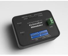
The Qi Receiver Simulator is a medium power receiver that can be used to test the operation and performance of Qi wireless power transmitters. DIP switches on top of the Qi Receiver Simulator can be used to select different operational test modes as well as select different communication modulators and internal loads.
