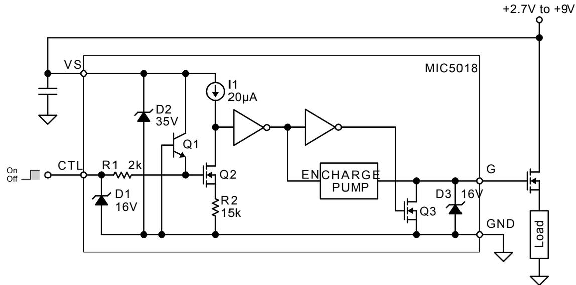
Functional Diagram with External Components
