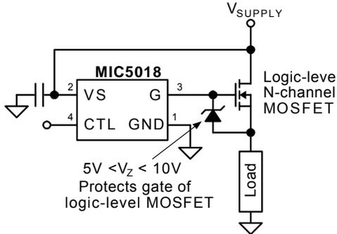
Figure 4. Gate-to-Source Protection
