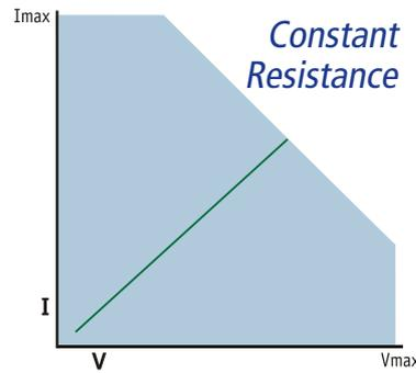
Constant resistance mode simulates a standard resistive load by providing a current drain proportional to voltage. Settings are displayed in Ohms or milli-Ohms.
