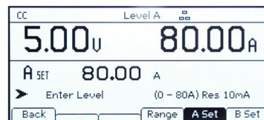
The meters have an accuracy of 0.1% for voltage and 0.2% for current.
