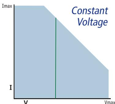
Constant voltage mode is used for load testing of constant current power supplies. The unit operates as a high power shunt regulator.
