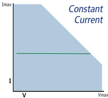
Constant current mode is used for load testing of normal voltage-source power supplies and for constant current discharge testing of batteries.
