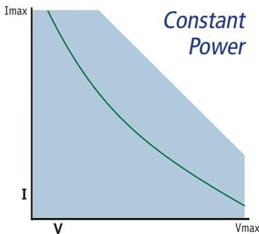
Constant power mode simulates a load whose power consumption is independent of the applied voltage. This is true of many types of equipment that incorporate switch-mode regulators. This mode may be particularly suitable for testing power sources of portable devices such as Lithium-ion batteries.
