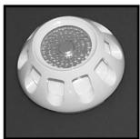
The BF302NEH fixed temperature heat detector incorporates a self-resetting bimetallic disk element with response indicator. It activates whenever the ambient air temperature reaches the top temperature setting of 70°C. The BF302NEH is generally suitable for areas such as boiler houses where temperatures rise too quickly for the reliability of rate of rise detectors. A red fire LED indicator is included and the detector is suitable for use with the BF318 remote LED indicator.
