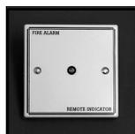
The BF318 Remote LED connects to the BF308N standard mounting base to indicate an alarm condition at detectors which are out of sight (in lift shafts, hotel bedrooms, behind false ceilings, etc). With a voltage range of 3 to 30 V dc, a high brightness LED and reverse polarity protection, the BF318 can also be connected directly to the sounder output of an alarm system as a visual indication. The white plastic case is 84mm square, 13mm deep and fits on a standard UK single gang back box.
