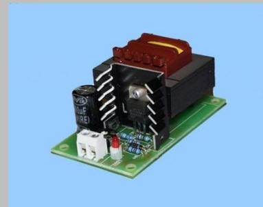
**Note:** The card must be mounted to provide adequate insulation requirements for the application. Attention should be paid to allowing sufficient cooling/ ventilation around the pcb in all eventualities of operation. The heatsink can get very hot.
