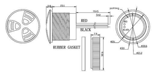
Dimensions : Millimetres Tolerance: ±0.5mm
