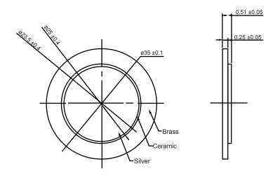
Dimensions : Millimeters Tolerance : ±0.5mm
