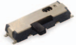
JSM08022SAQNL SPDT Surface Mount Momentary only
