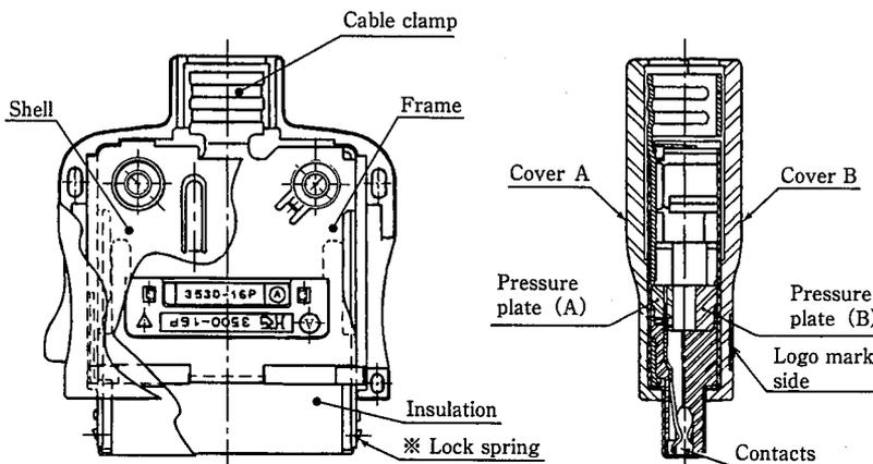
※ This lock spring forms a single body structure with the frame and cable clamp.
