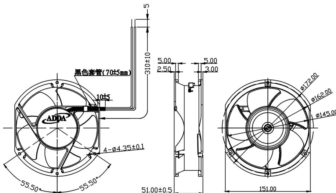
LEAD WIRES : UL 1061, AWG22 , L = 310±10 mm
