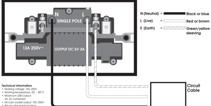
• Fits any standard backbox (minimum depth of 25mm).
