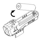
4. Ensure the battery cover is aligned properly on the LED probe clip light. Reverse the sliding direction to close the battery cover.
