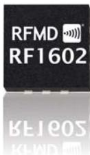
Package: QFN, 2mm x 2mm x 0.55mm
