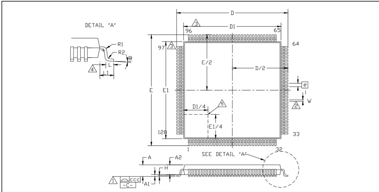
Figure 15.1 128 Pin TQFP Package Outline, 14X14X1.0 Body
