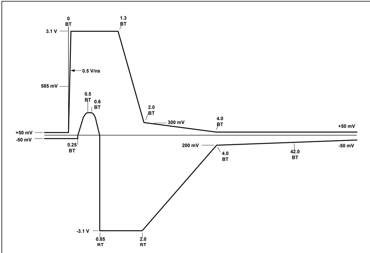
**Figure 7.7 Link Pulse Output Voltage Template - NLP, FLP**
