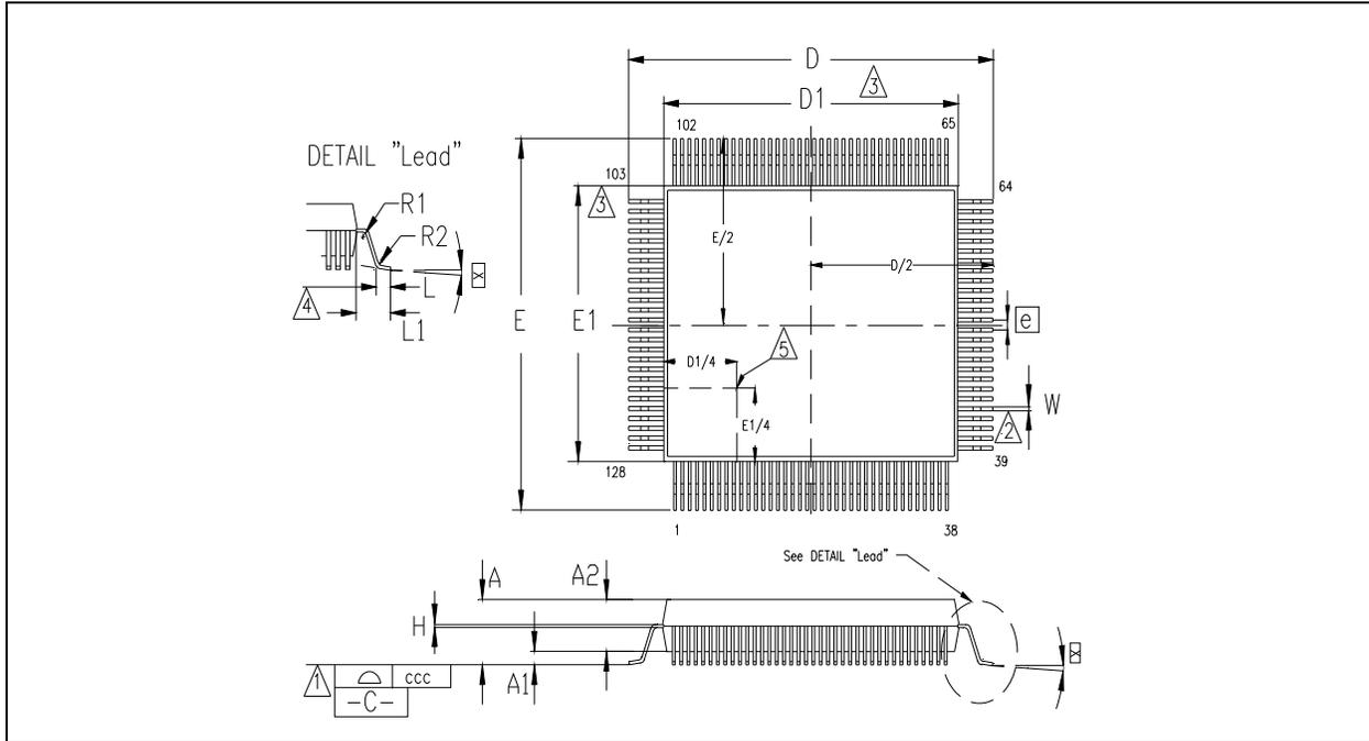
**Figure 15.2 128 Pin QFP Package Outline, 3.9 MM Footprint**
