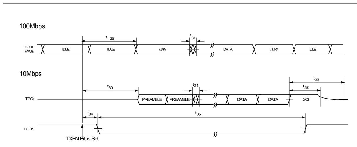
Figure 14.11 Transmit Timing
