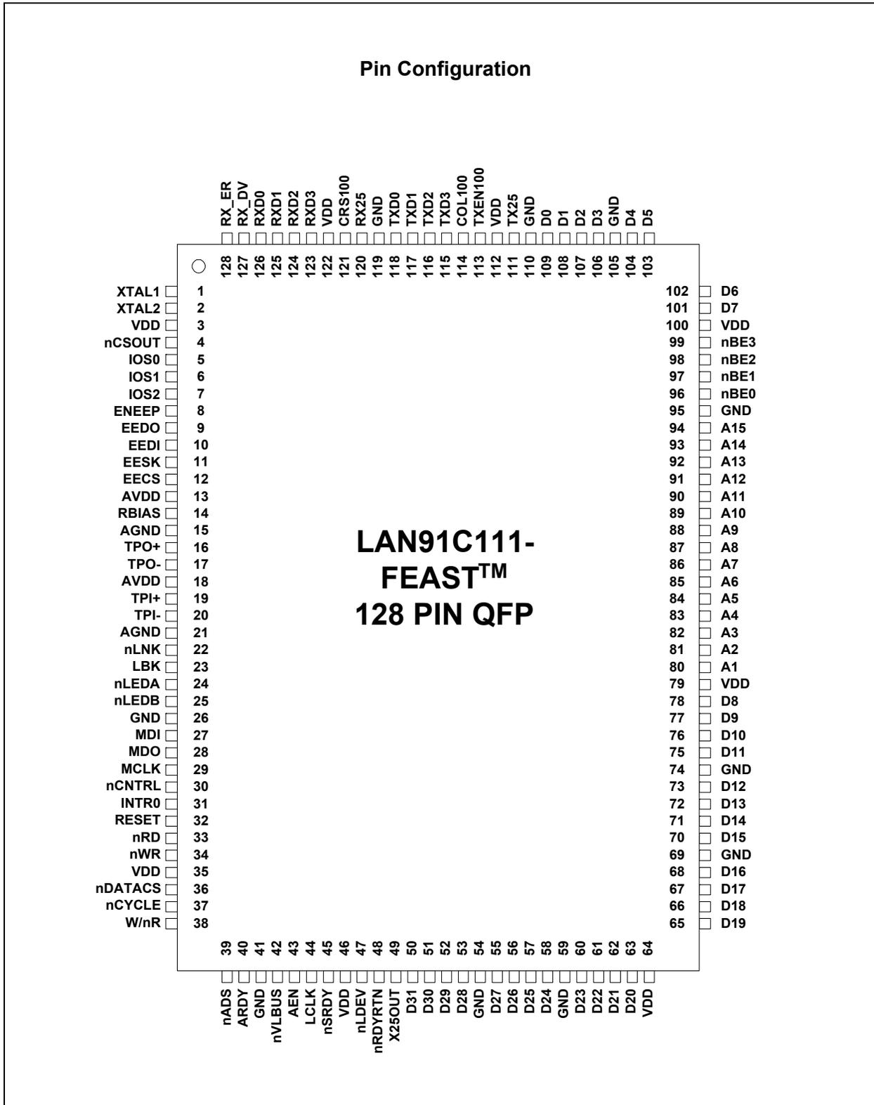
Figure 2.2 Pin Configuration - LAN91C111-FEAST 128 PIN QFP
