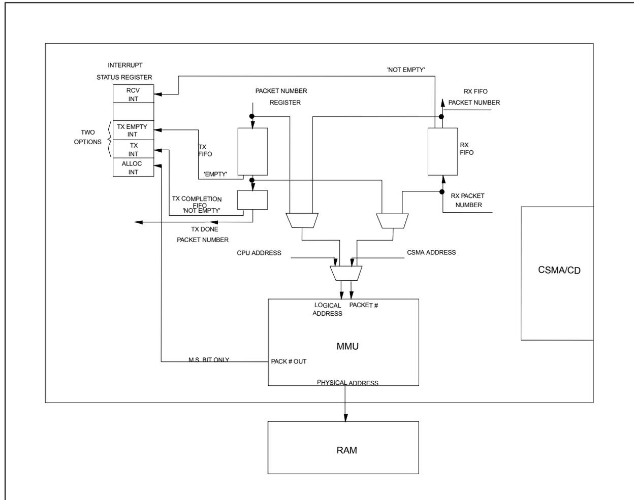
Figure 10.6 Interrupt Generation for Transmit, Receive, MMU
