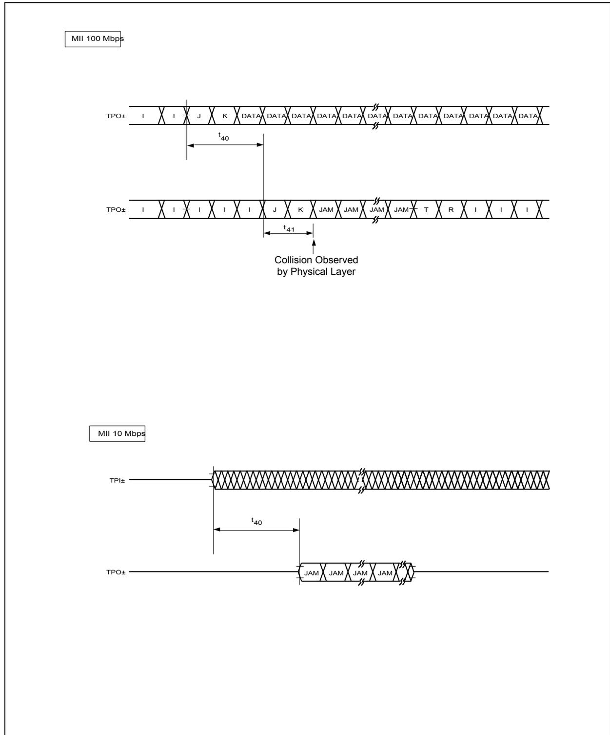
Figure 14.15 Jam Timing
