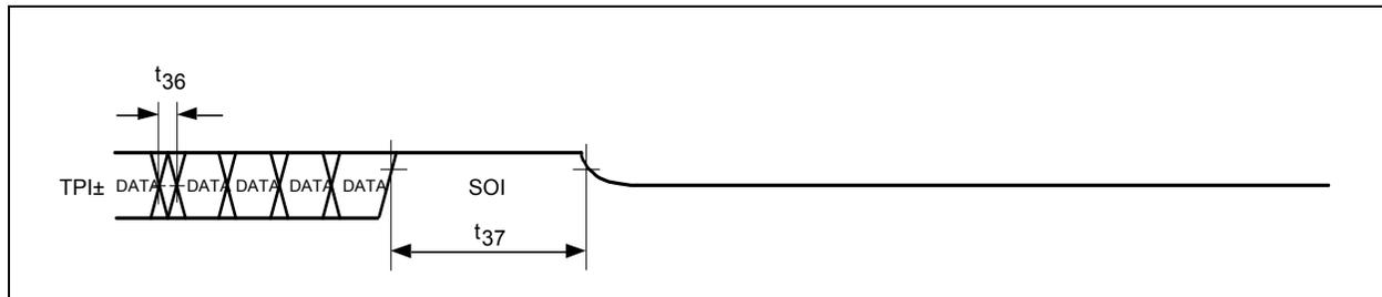
**Figure 14.12 Receive Timing, End of Packet - 10 MBPS**
