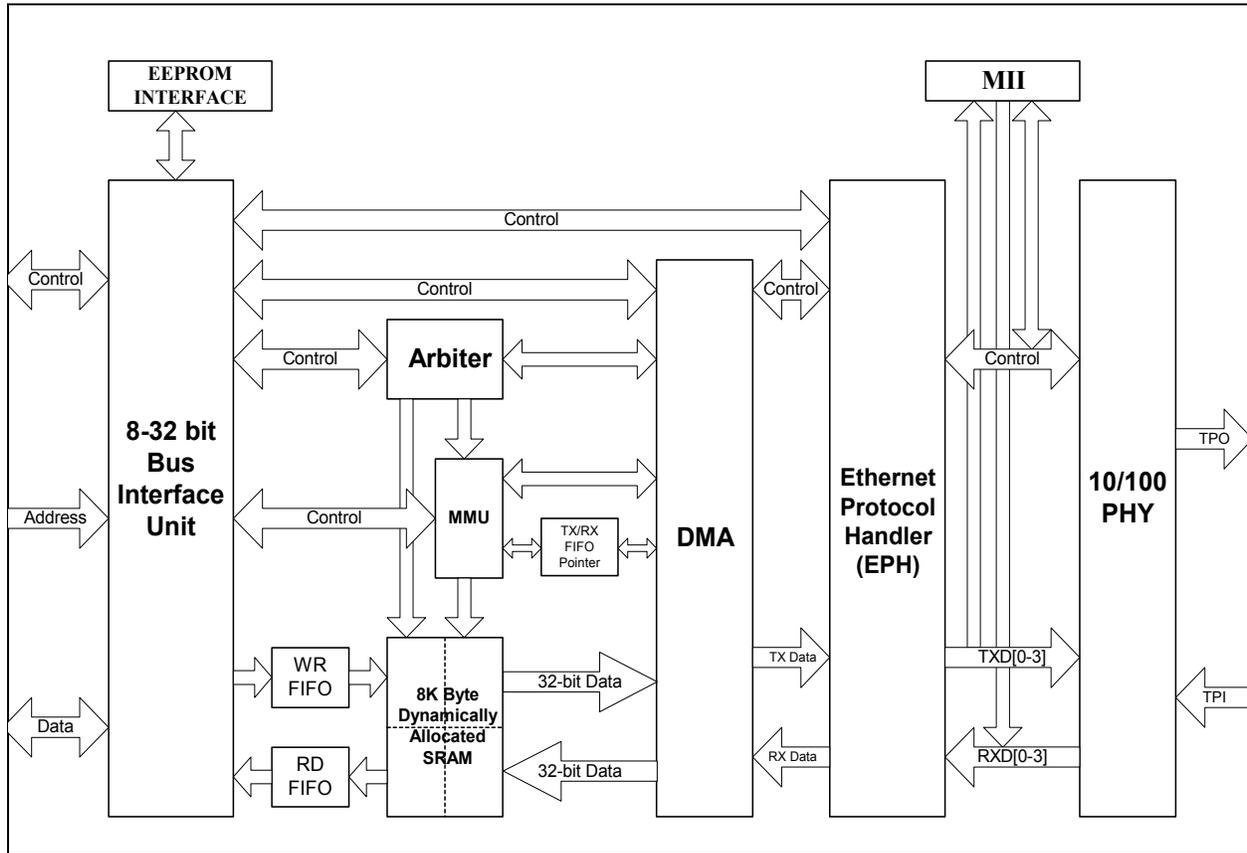
**Figure 3.2 Block Diagram**
