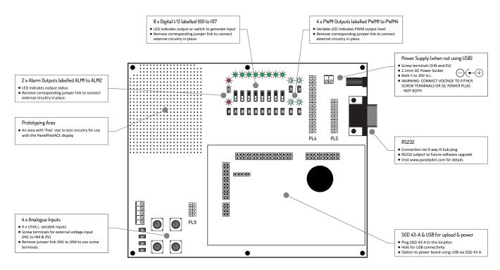
The main connection is that of the SGD 43-A supplied as part of the SGD 43-A-DK+ development kit. The board can be powered directly by connecting a USB cable to the rear of the display. Whilst connected the USB will provide power to both the display and the development board.
