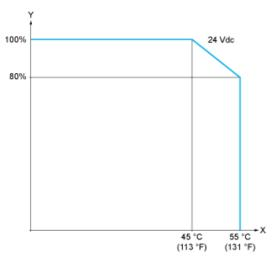
X: Ambient temperatureY: Input simultaneous ON ratio
