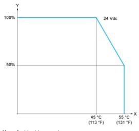
X: Ambient temperatureY: Input simultaneous ON ratio
