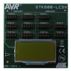
The STK600-LCDx is a breakout board for a 160 segment LCD display. It is used together with the STK600 and an ATxmega MCU w/ LCD driving capabilities.
