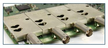
Careful front-end design and shielding reduces noise, crosstalk and harmonic distortion. Years of oscilloscope experience leads to improved pulse response and bandwidth flatness.
