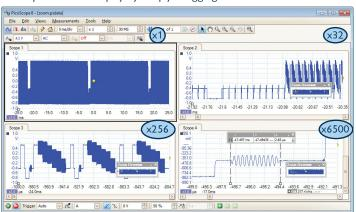
The deep memory can be segmented to store multiple waveforms, and has navigation tools allowing you to review up to 10,000 previous entries. No longer will you see a glitch on the screen only for it to vanish before you stop the scope. A mask can be applied to filter out waveforms of interest.
