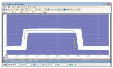
The numerical and graphical mask editors can be used separately or in combination, allowing you to enter accurate mask specifications and to modify existing masks. You can import and export masks as files.
