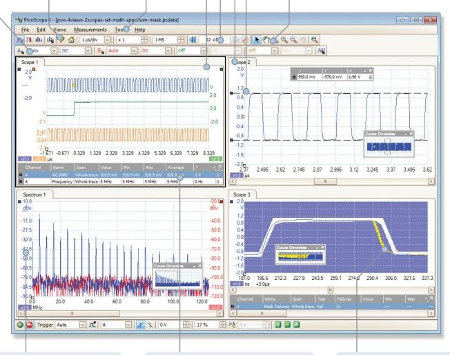
Movable axes: The vertical axes can be dragged up and down. This feature is particularly useful when one waveform is obscuring another. There's also an Auto Arrange Axes command.
