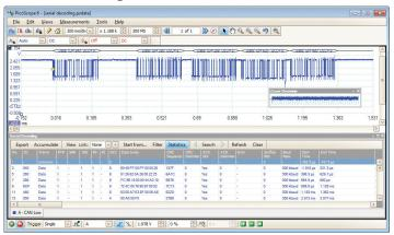
The deep-memory PicoScope 3000 Series is ideal for serial decoding as it can capture thousands of frames of uninterrupted data.
