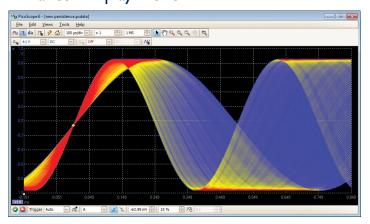
See old and new data superimposed, with new data in a brighter color or shade. This makes it easy to see glitches and dropouts and to estimate their relative frequency. Choose between analog persistence and digital color, or create a custom display mode.
