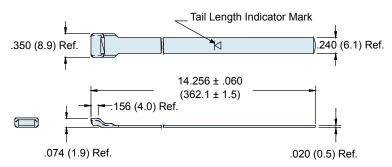
The 600-052 Standard Band is precision constructed of 300 Series SST/Passivate and designed for use with the 600-058 Hand Banding Tool or the 600-067 Pneumatic Banding Tool. Double-wrapped bands will accommodate diameters up to approximately 1.8 inches (45.7). Bands may be ordered flat (600-052) or precoiled (600-052-1). Bands come bagged and tagged in quantities from 1 to 100.
