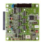
When connected to a DC9003A-B Evaluation/Development Mote, the **DC9006 Eterna interface card** provides a USB connection for both power and software access to the mote API UART port.
