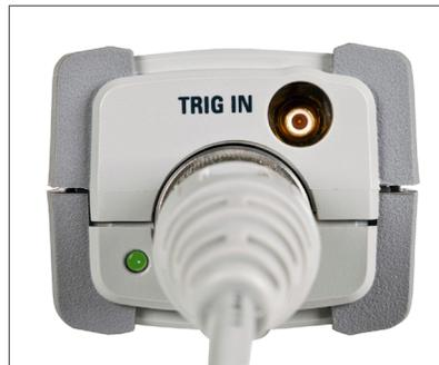
The external trigger input port on the U8481A.
