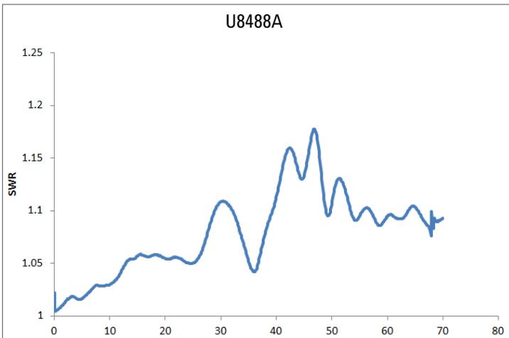
Figure 7. Typical SWR for the AC-coupled U8488A (Option 100)
