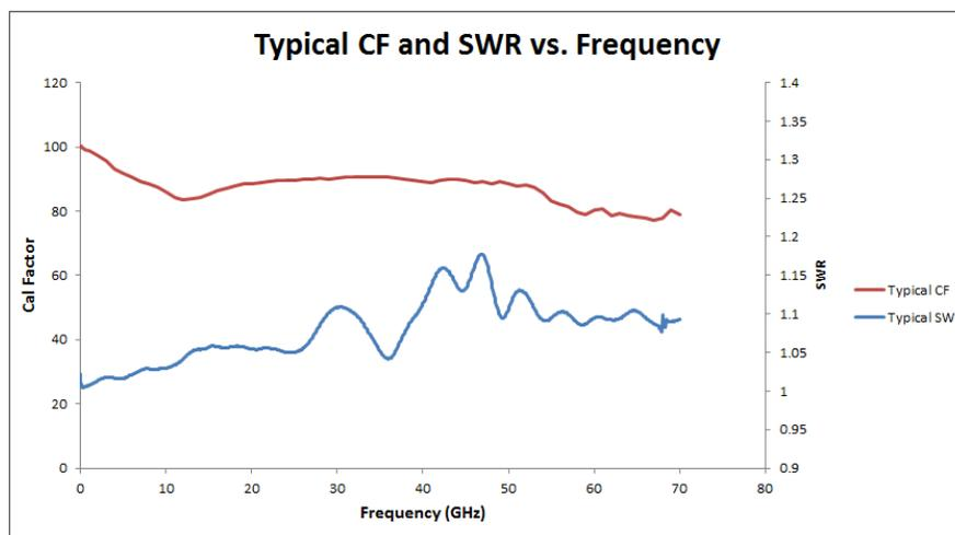
Figure 9. Typical calibration factor (CF) and SWR vs. frequency
