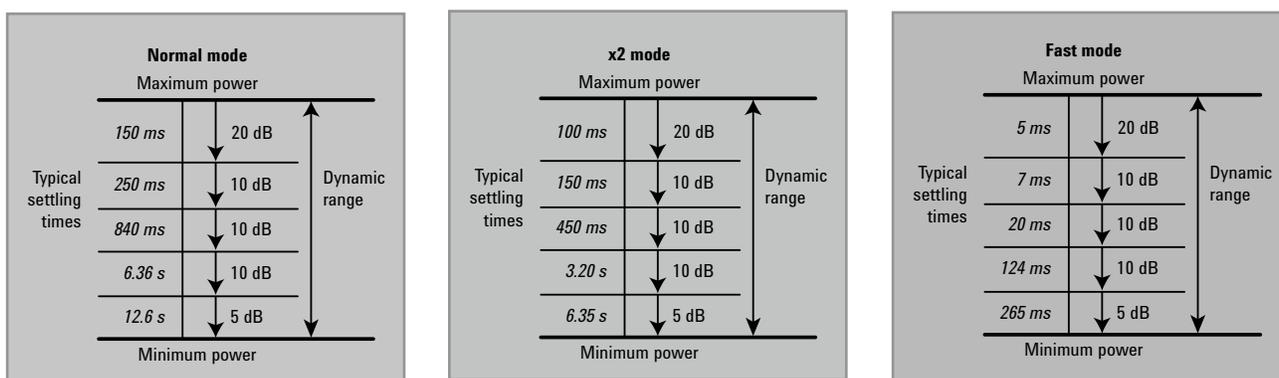
Figure 8. Auto-filter, default resolution, 10 dB decreasing power step
