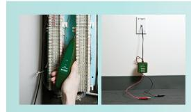
Non-Contact probe audibly identifies selected wire or cable. Easily trace wires from source to termination.
