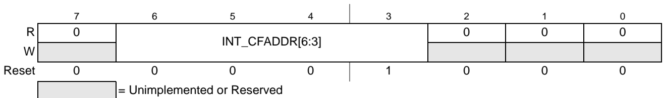
Figure 4-4. Interrupt Configuration Address Register (INT_CFADDR)
