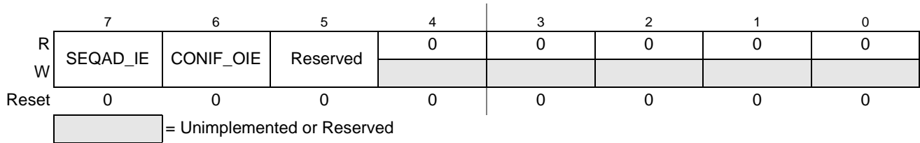
Figure 10-11. ADC Interrupt Enable Register (ADCIE)
