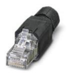
RJ45 connector, IP20, CAT5e, 8-pos., with QUICKON fast connection technology, for 1-wire and 7-wire conductors AWG 26 ... 22, for cable diameter of 4.5 mm ... 8.0 mm, TIA 568 B labeling, color: black
