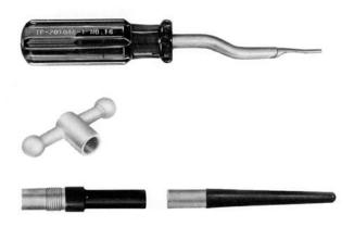
A separate expander barrel is required for each cavity of the contact inset.
