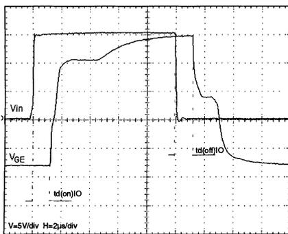
Fig. 11 Input and output voltage propagation time
