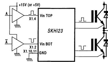
Fig. 4a Connecting the SKHI 23 with short cables
