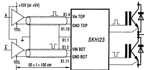
Fig. 4b Connecting the SKHI 23 with long cables
