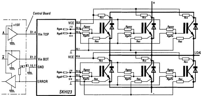
Fig. 10 Preferred circuit for parallel dual IGBT-modules
