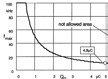
Fig. 15 Maximum operating frequency x gate charge
