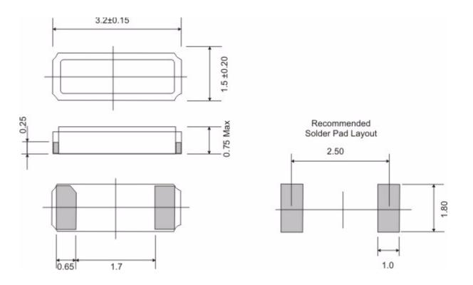
Holder Style Mode Adjustment Tolerance Operating Temp. Range Load Capacitance ESR Drive Level Ageing Marking 3,2 x 1,5mm Fundamental ± 20PPM at 25°C -40°C to +85°C 12.5 pF 80000 Ohm 1.0 uW mW +/-5ppm 1st Year Max DA\*\*\*C, D=Facory,A=32.768kHz,\*\*\* = lot No,C =China
