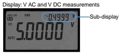
Display: V AC and V DC measurements
