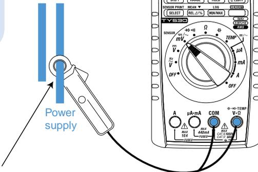
AC/DC clamp-on probe (Model 96095)
