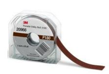
3M<sup>™</sup> Portable Utility Cloth Roll 314D is a versatile lightweight cloth abrasive sheet used on metal, wood, and plastic for either hand or machine sanding. These sheets are ideal for multiple metalworking applications on both ferrous and non-ferrous metals: deburring, blending and repairing metal finishes, rust or other contaminant removal, and surface preparation for paints and coatings.
