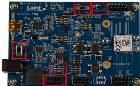
Figure 1: Switch and jumpers position
