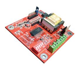
The DC temperature controller provides closed loop, temperature sensitive speed control for ebm-papst 2-wire and 3-wire DC fans. The controller regulates the electrical power supplied to the fan to maintain optimum performance and reliability.
