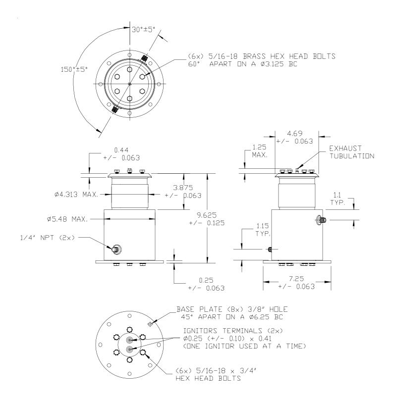
NOTE: The mounting flange attached to the bottom of the tube can be modified in most cases for compatibility with the users socket. In all cases coaxial returns "squirrel cages" are recommended. The anode contact must NOT be ridged with respect to the cathode and the flexible anode connection MUST absorb all buss bar movement.
