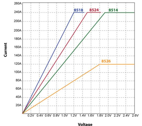
Typical minimum operating voltage at full scale current:
