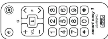
2. Press \* + # on the transmitter simultaneously for min. 3 seconds. Red LED lights on permanently.
