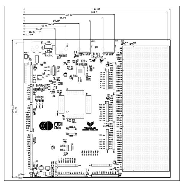
Dimensions in mm. Tolerance is  $\pm 0.1$ mm
