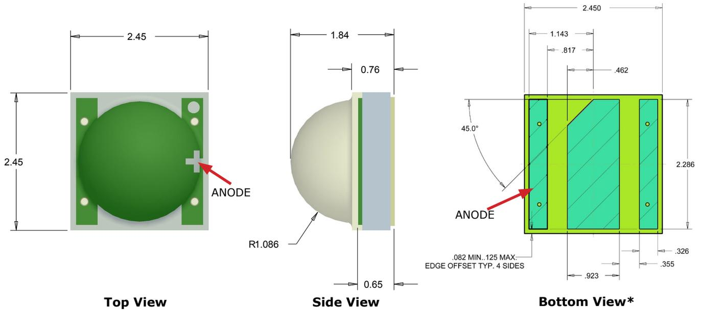
\* Note: In December, 2012, Cree changed the thermal pad of the XB-D package to include the anode notch illustrated above. XB-D LEDs produced prior to implementation of this change may have a different visual appearance.
