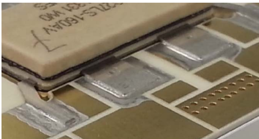
Fig 28. Wetting appearance (Pb-free solder joints)
